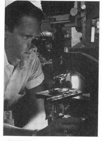
MULTIPLE BEAM INTERFEROMEIRY TECHNIQUE is used by B. D. Shafer (1433-2) to measure thin film thickness. Thin film laboratory is located in Bldg. 828.
